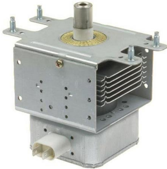
Magnétron 2.45 GHz, 1.2 kW (4.5 kV, 0.4 A, \eta = 60\% )
